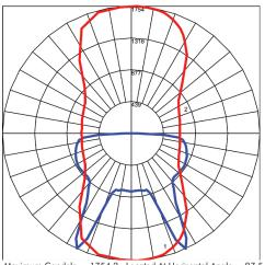
Maximum Candela = 1754.2 Located At Horizontal Angle = 87.5, Vertical Angle = 25 # 1 - Vertical Plane Through Horizontal Angles (87.5 - 267.5) (Through Max. Cd.) # 2 - Horizontal Cone Through Vertical Angle (25) (Through Max. Cd.)
