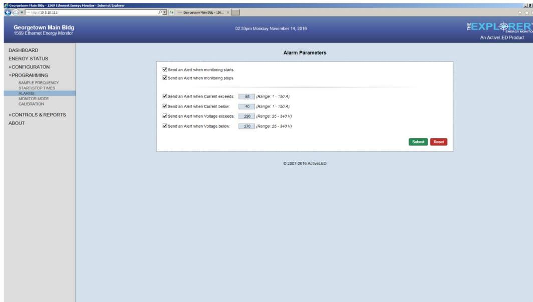
Set options to be notified by an Alarm. Alarm parameters include: Monitor start/stops, if Current exceeds or falls below a user specified range, and if Voltage exceeds or falls below set range. Notifications, or Alerts, will be sent to the specified email.
