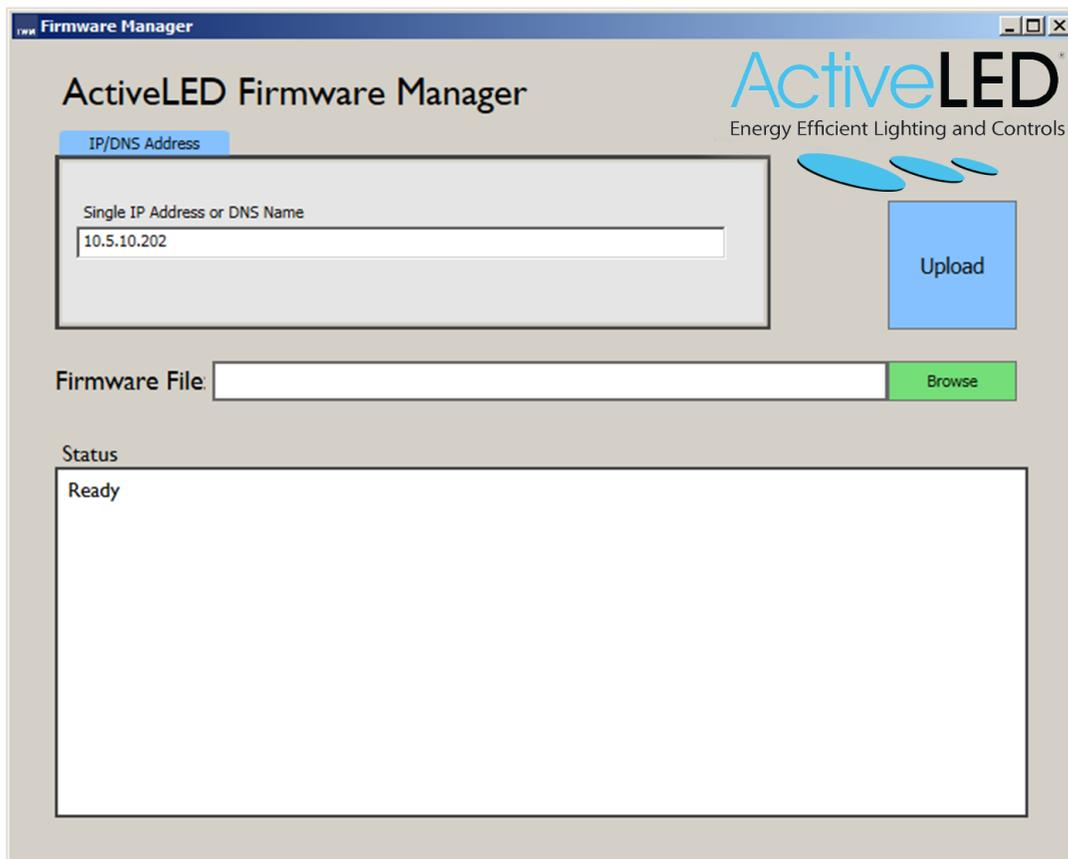
To upload firmware press the **Browse** button and select the Firmware (.dld) file. After the file is selected, upload the file by pressing the **Upload** button.
