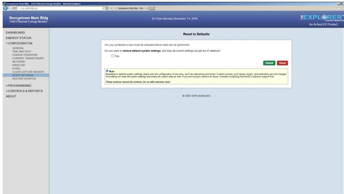
This will normally only be used under the direction of Technical Support. It will not change the IP Address of the Explorer Energy Monitor.
