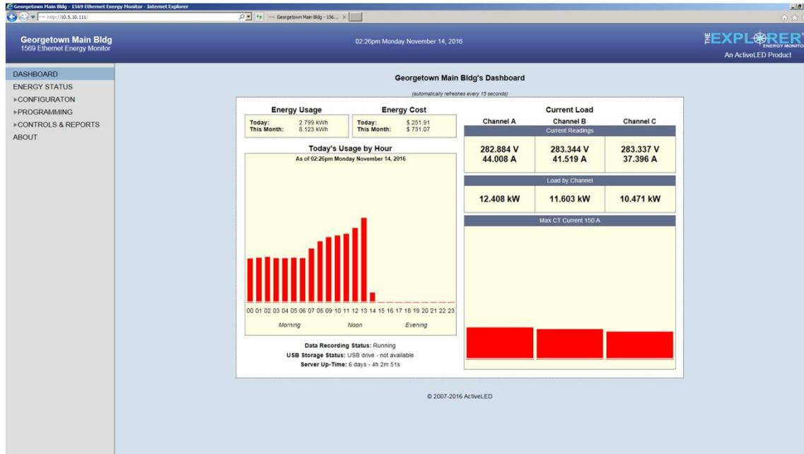
The upper panel shows the device description and the name currently assigned to the device – “Georgetown Main Bldg's Dashboard” in our example. The Dashboard also gives a quick view of energy usage in KWh and Cost as well as shows the days usage, broken down into 24 hours, and the Current Load.
