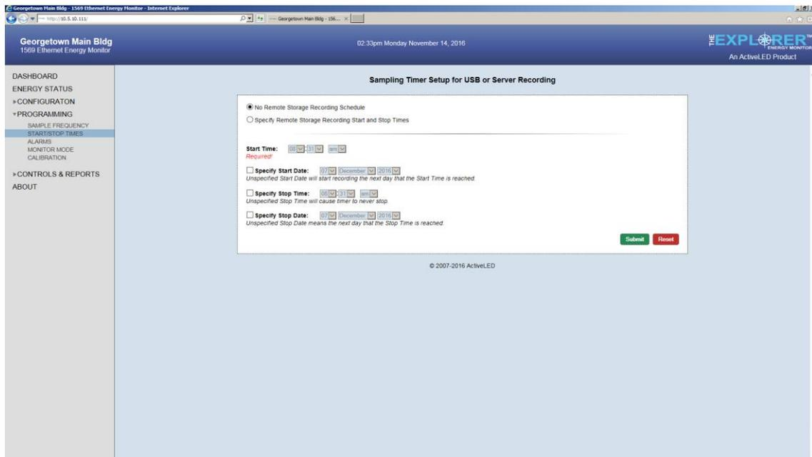
Each of the Start and Stop Times, Start Date and Stop Date may be given a value or left undefined. Leave all of these values undefined if you intend to start and stop the device manually.
