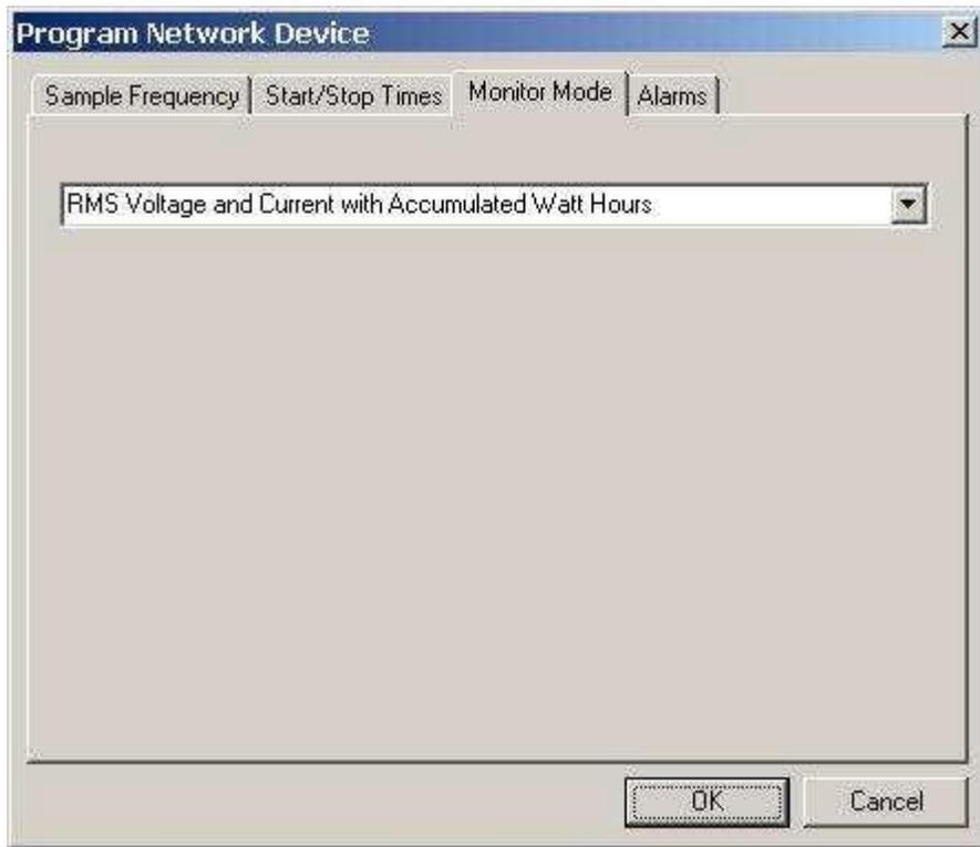
The initial option is RMS Voltage and Current with Accumulated Watt Hours. Other Monitor Mode options may be available by requesting through Technical Support. Email [support@ActiveLED.com](mailto:support@ActiveLED.com).
