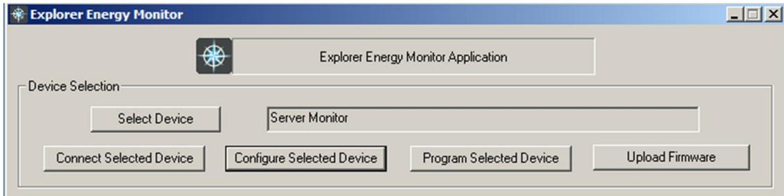
Once selected, the device's name will appear in the main panel and the three options "Connect Selected Device", "Configure Selected Device", and "Program Selected Device" will become available.
