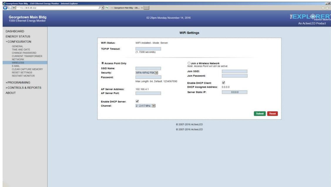
Wi-Fi Status - Displays if Wi-Fi is installed or not.
