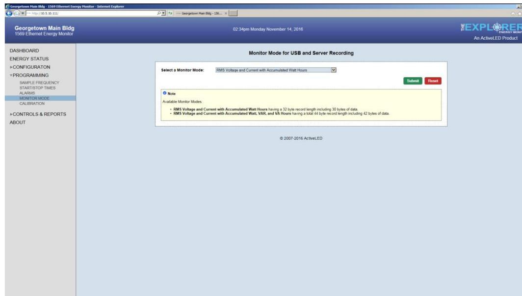
There are two fundamental monitor modes the first being the smallest record size recording only the basic information of voltage, current and watt hours occupying 32 bytes per record and thus allowing to store the maximum amount of records on the USB Flash drive. The extended mode records in addition reactive power and VA.
