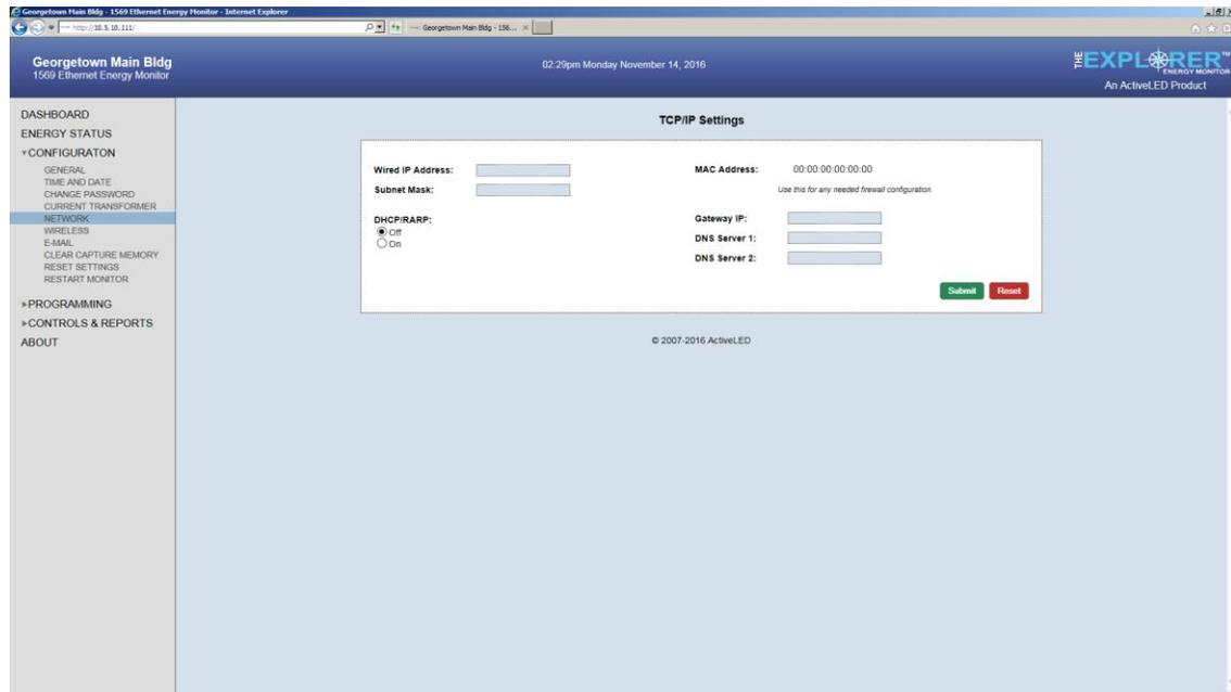
IP Address – Enter an unused IP Address from your network, or click on the DHCP/RARP Enable.
