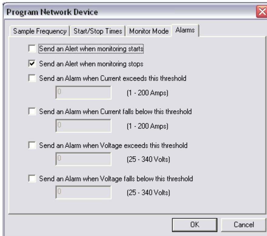
You can set an Alert to be sent to the Destination Email Address when monitoring starts and/or stops. Future revisions will current/voltage threshold triggers.
