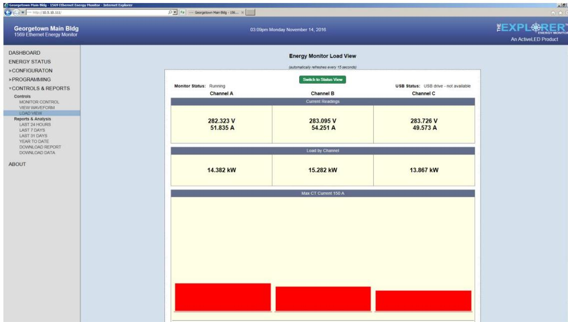
Load View displays the current energy usage, for separate channels, in voltage and amperage, and kW
