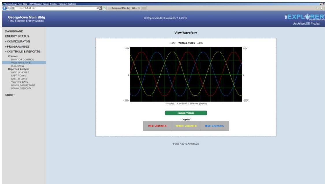
Sample Voltage - Used to view the Voltage waveform for each channel
