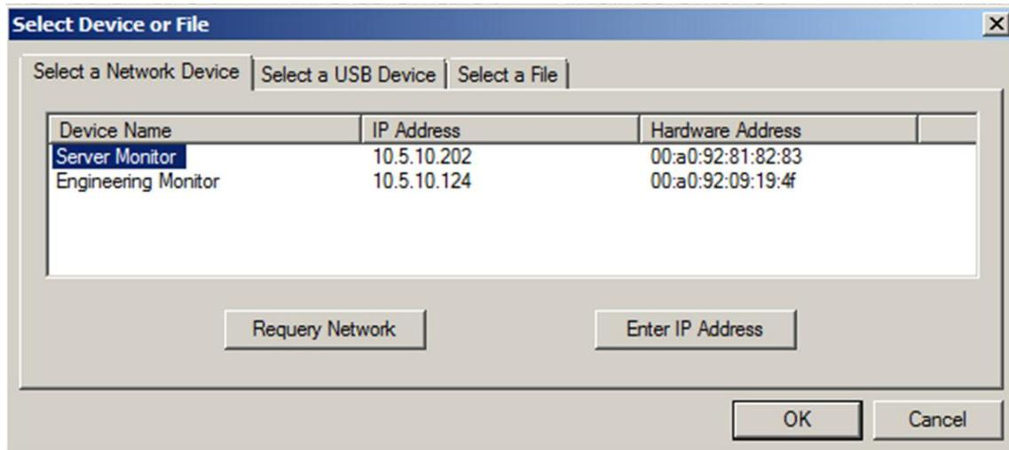
Any Explorer Energy Monitors on your network will show up in the panel as shown above. If it doesn't appear straight away, use the Requery Network button to try again to find the device. Click on the device that is to be configured to highlight it and then click the **OK** button.
